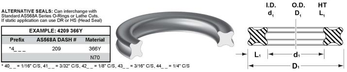
Quad rings are four-lobed seals that provide twice the sealing surface of an o-ring. They are free of mold parting lines (flash) or blemishes on those surfaces. The quad design resists spiral twist as is common with o-rings in reciprocating situations. Standard material is 70 durometer nitrile. Other materials available upon request.
